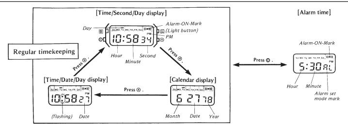
In the alarm time mode, the alarm-ON-mark disappears (the alarm is released) or appears each time the D button is pressed.
