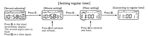
(Independent correction) Correction of any digit, if not required, can be skipped by pressing the ® button repeatedly in time/calendar/alarm setting.
