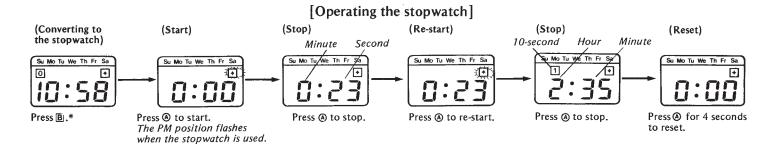
\* When the display is other than 0:00, press the @ button for 2 seconds or more until 0:00 is displayed.
