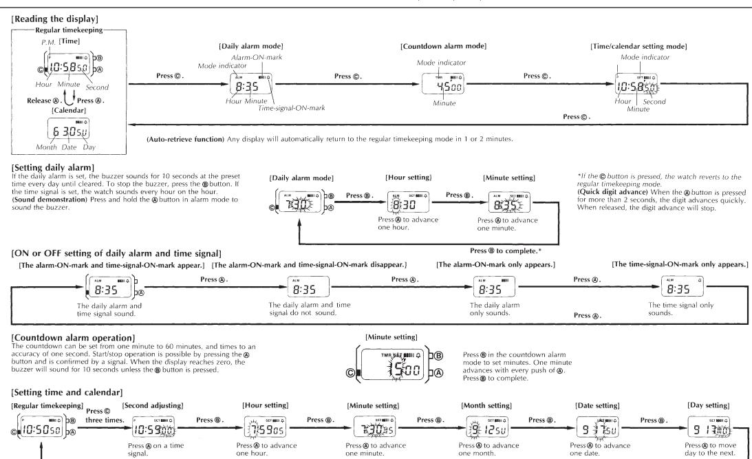
(Quick digit advance) When the ® button is pressed for more than 2 seconds, the digit advances quickly, When released, the digit advance will stop. (Independent correction) Correction of any digit, if not required, can be skipped by pressing the ® button repeatedly. (Auto-retrieve function) Any setting display will automatically return to the regular timekeeping mode in 1 or 2 minutes.
