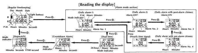
(Changeover between 12-hour and 24-hour formats) In regular time keeping and dual time modes, with every push of (a), the display is switched between 12-hour and 24-hour formats.
